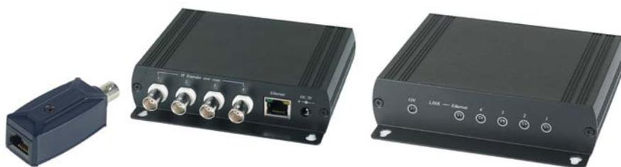
IP01 is a low cost and easy, speedy solution to allow you use existing coax cable to send IP camera signal. Used in pairs with your RG59 cable to exceed the IEEE 802.3 10BaseT specification. The working range could up to 200 meters at 10Mbps speed.
